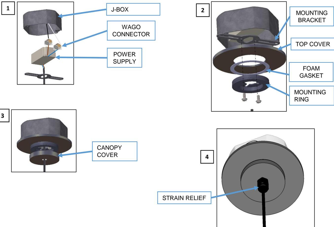
1. ADJUST THE CORD LENGTH ,LOOSE THE STRAIN RELIEF ON THE COVER AND MOVE IT ALONG THE POWER CORD TO THE DESIRED HEIGHT. CUT AND STRIP THE CABLE TO REVEAL 2 WIRES, STRIP THE 2 WIRES AND CONNECT TO THE MAIN LINE TO POWER SUPPLY USING THE WAGO CONNECTORS ALREADY ON THE FIXTURE, BROWN TO BLACK AND BLUE TO WHITE. (FIGURE 1)
